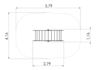
Critical fall height (CFH) A1: CFH 1,0m - 21,17m<sup>2</sup> Rubber surface area - 21,17m<sup>2</sup> Tatal area: 21,17m<sup>2</sup>
