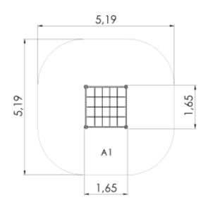
Critical fall height(CFH) A1: CFH 1,92m - 24,25m<sup>3</sup> Rubber surface area - 24,25m<sup>3</sup> Total area: 24,25m<sup>3</sup>
