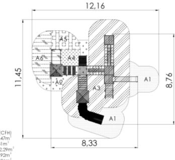
Critical fall height(CFH) A1: CFH 1.0m - 17.47m<sup>2</sup> A2: CFH 1.2m - 8.31m<sup>2</sup> A3: CFH 1.55m - 42.29m<sup>2</sup> A4: CFH 1.67m - 2.92m<sup>2</sup> A5: CFH 1.79m - 4.36m<sup>2</sup> A6: CFH 1.92m - 9.53m<sup>2</sup> Rubber surface area - 84.88m<sup>2</sup> Total area: 84.88m<sup>2</sup>
