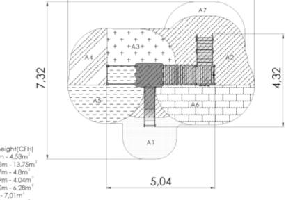
Critical fall height(CFH) A1: CFH 1.0m - 4.53m<sup>2</sup> A2: CFH 1.55m - 13.75m<sup>2</sup> A3: CFH 1.67m - 4.8m<sup>2</sup> A4: CFH 1.79m - 4.04m<sup>2</sup> A5: CFH 1.92m - 4.28m<sup>2</sup> A6: CFH 2m - 7.01m<sup>2</sup> A7: CFH 0.6m - 2.41m<sup>2</sup> Rubber surface area - 40.41m<sup>2</sup> Total area: 42.82m<sup>3</sup>
