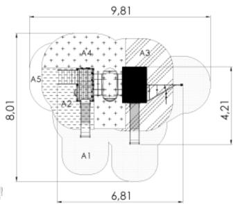
Critical fall height(CFH) A1: CFH 1,0m - 18,67m<sup>2</sup> A2: CFH 1,2m - 8,17m<sup>2</sup> A3: CFH 1,55m - 11,73m<sup>2</sup> A4: CFH 1,98m - 13,16m<sup>2</sup> A5: CFH 0.6m - 2.14m<sup>2</sup> Rubber surface area - 51.73m<sup>2</sup> Total area: 53.87m<sup>2</sup>
