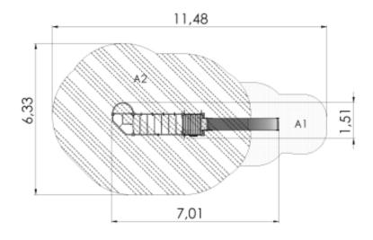
Critical fall height(CFH) A1: CFH 1.0m - 8.78m<sup>2</sup> A2: CFH 2.95m - 42.13m<sup>2</sup> Rubber surface area - 50.91m<sup>2</sup> Total area: 50.91m<sup>2</sup>
