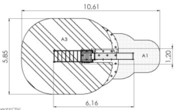
Critical fall height[CPH] A1: Criti 1,0m - 6,76m A2: Criti 2,15m - 4,1m A3: Criti 2,915m - 33,3m Rubber surface area - m Total area: 46,18m
