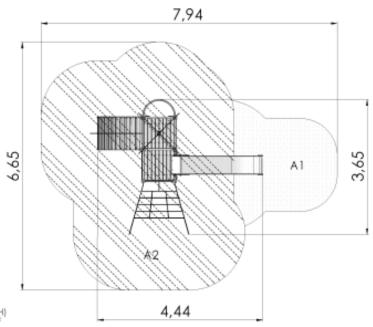
Critical fall height(CFH) A1: CFH 1.0m - 6.88m<sup>2</sup> A2: CFH 1.55m - 29.08m<sup>2</sup> Rubber surface area - 35,96m<sup>2</sup> Total area: 35,96m<sup>2</sup>
