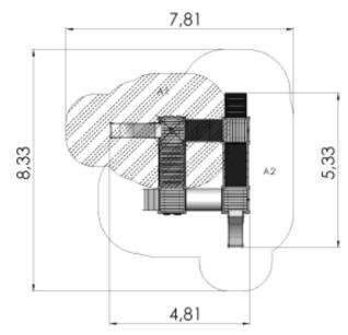
Critical fall height(CFH) A1: CFH 0,95m - 17,83m<sup>3</sup> A2: CFH 0,6m - 29,69m<sup>2</sup> Total area: 47,52m<sup>3</sup>
