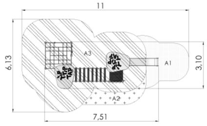
Critical fall height(CFH) A1: CFH 1.0m - 7.4m<sup>2</sup> A2: CFH 1.2m - 3.41m<sup>2</sup> A3: CFH 1.55m - 37.12m<sup>2</sup> Rubber surface area - 47.93m<sup>2</sup> Total area: 47.93m<sup>2</sup>
