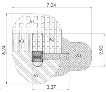
Critical fall height(CFH) A1: CFH 1.0m - 8,82m<sup>2</sup> A2: CFH 1.55m - 7,75m<sup>2</sup> A3: CFH 1.67m - 2,83m<sup>2</sup> A4: CFH 1.79m - 4,23m<sup>2</sup> A5: CFH 1,92m - 6,37m<sup>2</sup> Total area: 30m<sup>2</sup>
