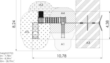
Critical fall height[CFH) A1: CFH 1,0m - 7,78m<sup>2</sup> A2: CFH 1,2m - 8,39m<sup>2</sup> A3: CFH 1,35m - 28,79m<sup>2</sup> A4: CFH 1,55m - 14,12m<sup>2</sup> A5: CFH 1,92m - 20,45m<sup>2</sup> Rubber surface area - 79,53m<sup>2</sup> Total area: 79,59m<sup>2</sup>
