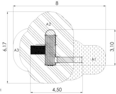
Critical fall height(CFH) A1: CFH 1.0m - 7.24m<sup>2</sup> A2: CFH 1.55m - 23,36m<sup>2</sup> A3: CFH 0.6m - 2,02m<sup>2</sup> Rubber surface area - 30,6m<sup>2</sup> Total area: 32,62m<sup>2</sup>
