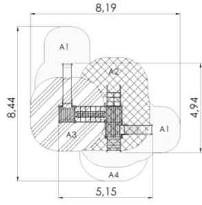
Critical fall height(CFH) A1: CFH 1,0m - 13,76m<sup>2</sup> A2: CFH 1,2m - 13,44m<sup>2</sup> A3: CFH 1,55m - 14,21m<sup>3</sup> A4: CFH 0,6m - 2,68m<sup>2</sup> Rubber surface area - 41,41m<sup>3</sup> Total area: 44,09m<sup>2</sup>
