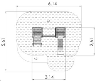
Critical fall height(CFH) A1: CFH 0.95m - 26.63m<sup>2</sup> A2: CFH 0.6m - 1.86m<sup>3</sup> Rubber surface area - 26.63m<sup>2</sup> Total area: 28.49m<sup>2</sup>
