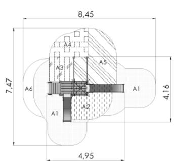
Crifical fall height (CFH) A1: CFH 1,0m - 16,92m<sup>2</sup> A2: CFH 1,2m - 5,64m<sup>2</sup> A3: CFH 1,5m - 2,4m<sup>2</sup> A4: CFH 1,67m - 3,5m<sup>2</sup> A5: CFH 1,92m - 7,17m<sup>2</sup> A6: CFH 0,67m - 2,38m<sup>2</sup>
