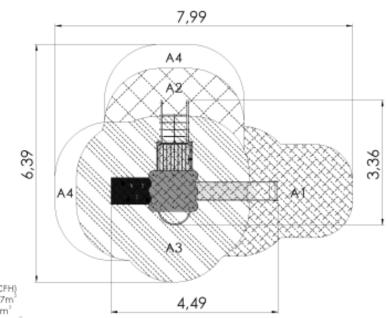
Critical fall height (CFH) A1: CFH 1,0m - 10,77m<sup>3</sup> A2: CFH 1,2m - 4,38m<sup>3</sup> A3: CFH 1,55m - 13,55m<sup>2</sup> A4: CFH 0.6m - 4.49m2 Rubber surface area - 28,7m² Total area; 33,19m²
