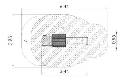
Critical fall height(CFH) A 1: CFH 0,95m - 18,05m<sup>2</sup> A2: CFH 0,6m - 2,66m<sup>2</sup> Total area: 20,71m<sup>2</sup>
