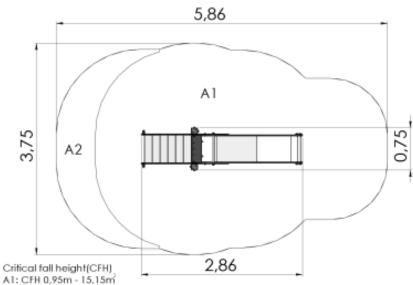
A1: CFH 0,95m - 15,15m A2: CFH 0,6m - 2,43m Rubber surface area - 15,15m²
